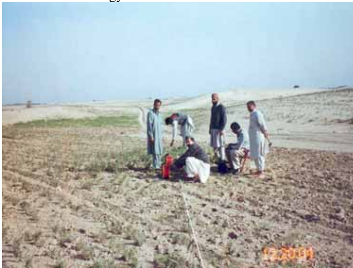
Electrical Resistivity Survey by ABEM Terrameter
