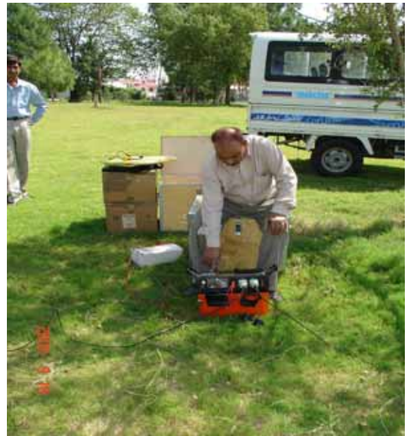
ABEM Seismograph for groundwater investigations
