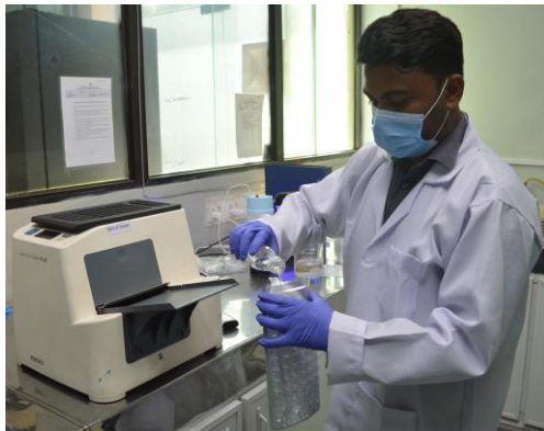
Figure 13: Mixing of Media with Sample; Pouring into Quanti tray
