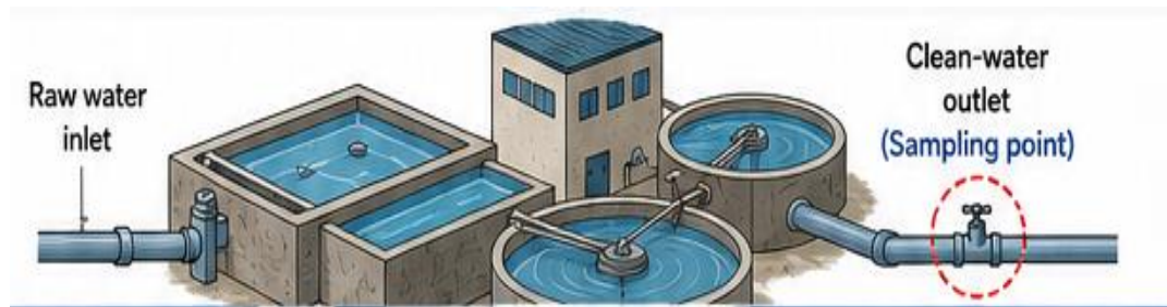
Figure 7: Treatment Plant Outlet Sampling
