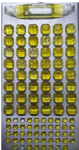
Figure 15: Count yellow wells as positive for "Total Coliforms"
