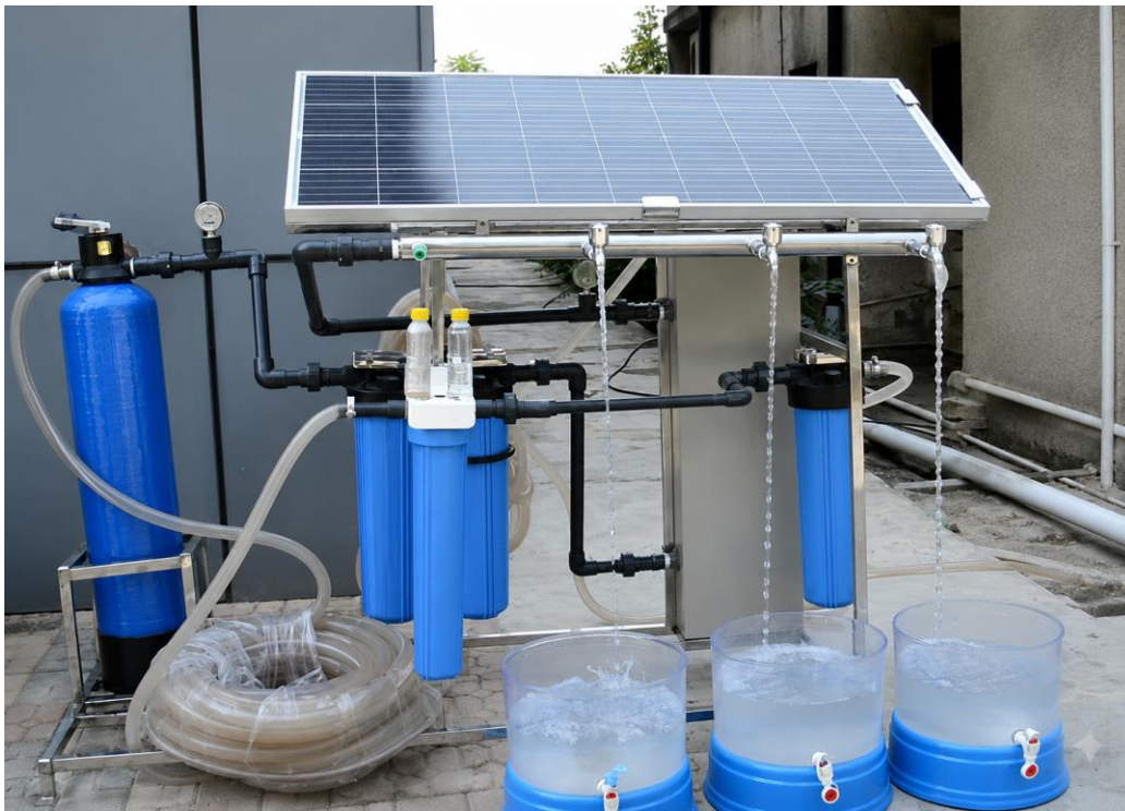
Figure 20: PCRWR Solar powered water filtration system
